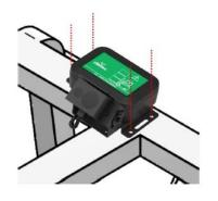
3. Fix the HLS sensor. Using an Allen key, tighten screws A and B.
