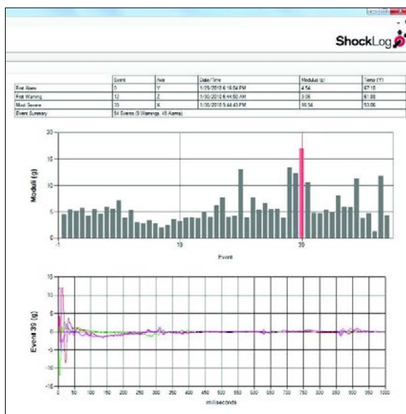
ShockLog software data (left) and optional SpotSee Cloud interface for monitoring real-time journey conditions – available with satellite or cellular modules (above).
