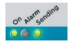
Alarm Triggered - When SpotBot experiences an impact above the "Alarm Threshold," the 'Alarm" (red) as well as the "On" and "Sending" (green) lights will flash at different intervals. The lights continue to flash as the SpotBot unit sends the alarm data to the SpotSee Cloud.
