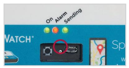
This action will clear all the data on the device and in the report tables, allowing you to start a new monitoring.
