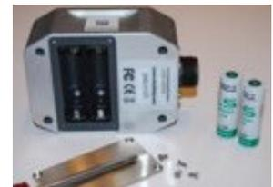
**Note:** All ShockLog units are rated to IP67. The battery compartment is isolated from the main body of the ShockLog unit and a poor fitting of the battery cover will not dramatically affect the IP rating of the main unit. However, if there is water ingress into the battery compartment, the batteries are likely to short and cause corrosion of the battery terminals. If this corrosion occurs, the ShockLog will not function correctly, and the unit will need to be returned to SpotSee for repair.
