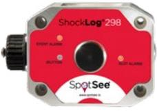
Avoid building special brackets to mount the ShockLog. If a cover is required, place the cover over the ShockLog but do not attach it to the ShockLog.
