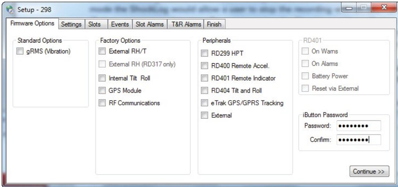
When a ShockLog is programmed with an iButton password, all iButtons used with that ShockLog unit must be programmed with the same password, otherwise the ShockLog unit will ignore the command. To program an iButton with the appropriate password, the iButton must be connected to the PC via the USB connection BUS and then the Password tab selected.
