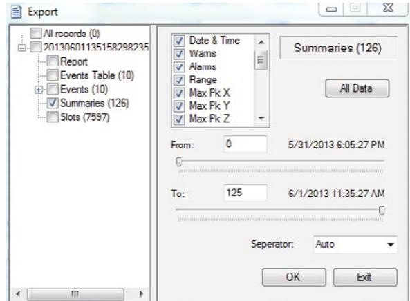
All these parameters are adjustable. For example, if there are channels of data that are not of interest simply uncheck the appropriate box. It is possible to use the slide bars to adjust the start and finish times of the data to be exported.
