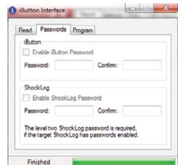
Once the password has been set, it is necessary to reprogram the iButtons by following the instructions in the “Program” section below.
