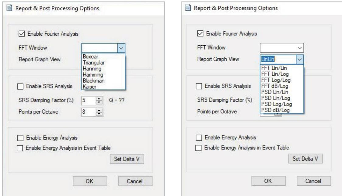
Scroll through the events until the event of interest is displayed. Turn the FFT or PSD analysis on by clicking FFT/PST Off and selecting the desired graph view. FFT Lin/Lin was selected for the image below:
