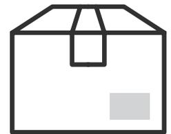
**Step 2:** If the package is twice as long as it is wide, use two ShockDot Impact Indicators. Place a second Indicator in the same position on the opposite side of the package.
