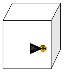
2. If the package is twice as long as it is wide, use two ShockWatch RFID Impact Indicators. Place a second indicator in the same position on the opposite side of the package.
