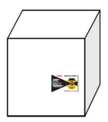
If the package is twice as long as it is wide, use two ShockWatch RFID Impact Indicators. Place a second indicator in the same position on the opposite side of the package.
