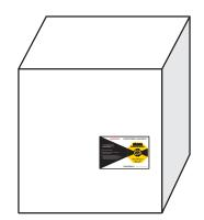
If the package is twice as long as it is wide, use two ShockWatch RFID Impact Indicators. Place a second indicator in the same position on the opposite side of the package.
