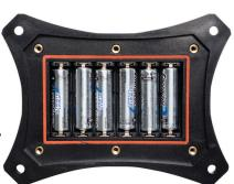
C. Install the (6) AA batteries provided in the direction notated within each battery slot and replace Battery Panel making sure that CE sticker is visible. Tighten the screws on the battery cover to a torgue setting of 116 -121 inch-ounces to preserve IP ratings
