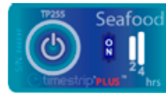
Armed: blister squeezed, the word "ON" will be visible and blue color change in the arming window confirms product is armed.
