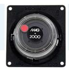
Your Shockwatch MAG2000 units may arrive in an activated condition, that is, with the red indicator showing (as shown left).
