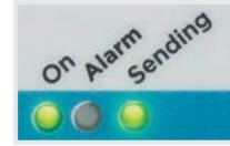
**B. In Use (No Alarm)** – When SpotBot is in use and not in process of sending an alarm to the SpotSee Cloud the “On” light will flash green every minute if no alarm has occurred. This light will flash yellow if the unit has low battery life remaining.
