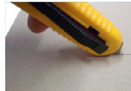
2. Release blade slider while cutting.
