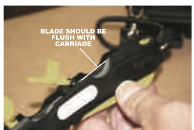
**CUTTER POSTURE:** <u>IMPORTANT</u>. Shown below is the correct way to hold the cutter when cutting. Squeeze the trigger to engage blade. Once
