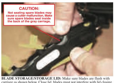
carriage as shown below. Close lid, blades must not interfere with lid closing.
