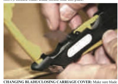
is flush with carriage as shown below. Close cover, blade must not interfere
