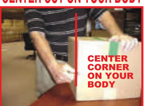
**TOP CUT:** Extend the edge guide. Using the proper cutting angle. Center box in front of you as shown in the inset picture. Engage blade and make
