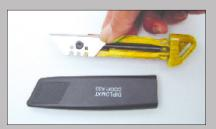
Replace blade and re-assemble knife. Then test safety knife operates correctly.
