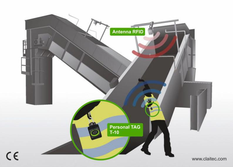
Claitec solution has been installed in hazardous areas of more than 110 recycling plants, protecting all workers in dangerous areas and falls onto conveyor belts, preventing serious accidents by automatic machine shutdown.
