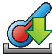
This is the **Current Tag Temperature** icon. Click while scanning or connected to view current temperature.
